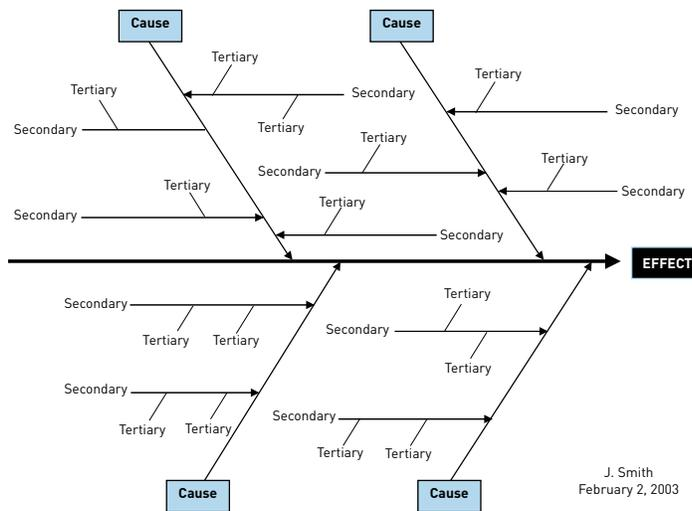
A **Cascade Diagram** is a tool that shows a cause-effect relationship. It starts with a statement of a problem/effect that is being investigated. A general cause of the problem is broken down to more specific causes that are then presented in the boxes. This is a visual tool that explores the specific roots of a problem through analysis of primary causes.
